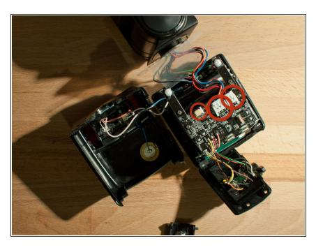
Remove the three wire harness plugs from their sockets on the PCB.
