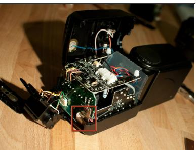
Remove the battery case unit (the battery case surrounded by 3 PCBs). The only thing keeping it in place is a single plug/socket at the bottom rear of the body and a bit of glue on hithe top. A spudger is useful here.
