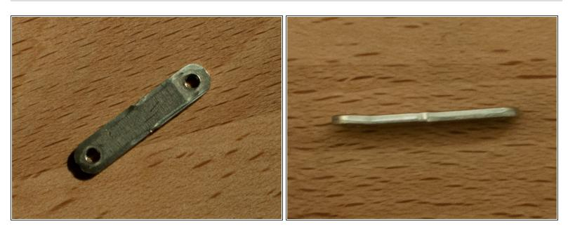
• When you were pulling it apart these things fell out, didn't they? They go in the 2 slots at the bottom of the body. The four screws on the leg unit screw into them. Make sure the screw holes line up before you put the whole case on. They have a slight bend on one end, and that end goes towards the back of the body (towards the LCD).
