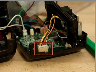
Remove the 5 wiring harnesses from their socket. I used a pair of needlenose pliers for the plug on the far left successfully (it has a lip that catches on the pliers) but I used the spudger for the rest.
