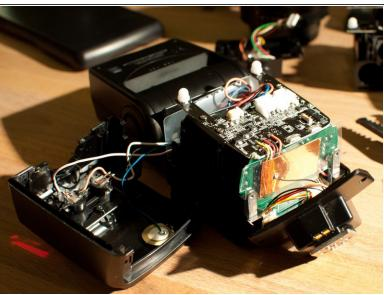
Undo the battery door and gently pull the front of the case off. It has wires connected to it so don't pull too hard.
