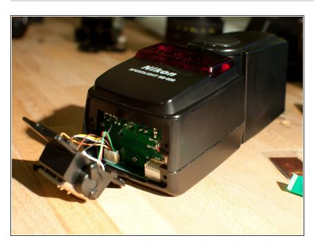
Pull leg unit from the bottom of the flash. Yours will look slightly different - there will be a copper plate inside that the leg unit is soldered to. Try not to tear it off or you will have to do some soldering.
