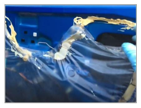
Remove the plastic cover from the inside of the door to access the interior mechanisms.
