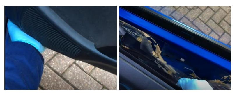
If the panel is press-fit onto the door, use your hands to un-clip the panel.
