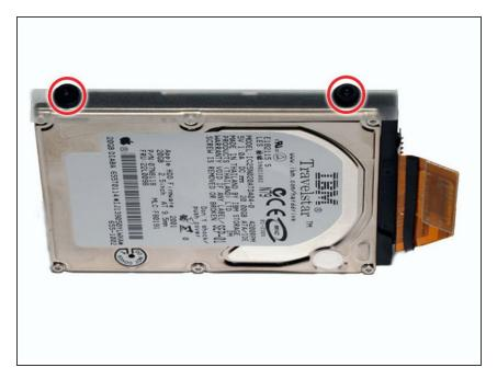
Remove the two black plastic bumpers and two T8 Torx screws from the side of the hard drive.
