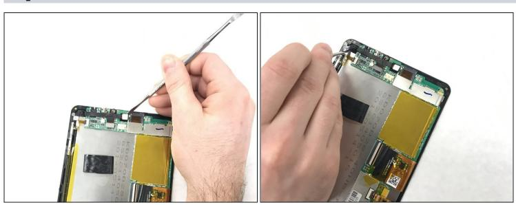
• Pry the connector that attaches the front and back camera with a metal spudger.
