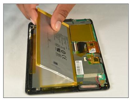
• Lift the battery from the device.
