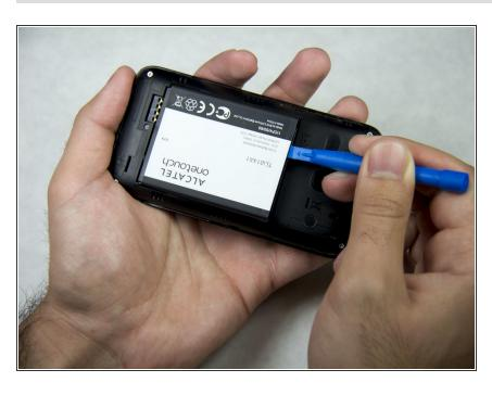
Remove the battery using one of the plastic opening tools and the domeshaped indent next to the battery face.
