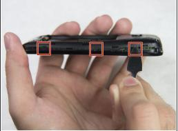
• Insert a plastic or metal spudger between the front cover and rear frame in one of the areas indicated by the red squares and gently pry the rear frame loose. Repeat the process all the way around the phone until the rear frame comes loose.
