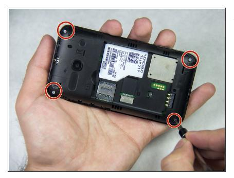
Unscrew the four 4mm JIS screws in each corner using the J000 screwdriver head. Turn the screws counter-clockwise to loosen.
