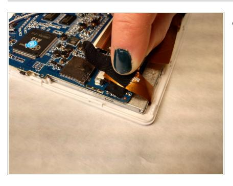
Remove black tape and using your fingers, pull the orange ribbon labeled BSR028-V3-KDX out of its port.
