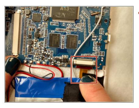
Remove the last orange ribbon labeled 24 by pulling the motherboard away from the ribbon
