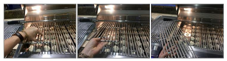
Carefully lift grill plate located above briquettes
