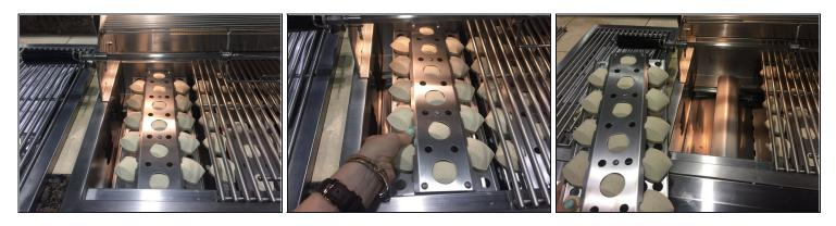
• Carefully remove entire ceramic briquette casing from above the stainless steel burner.
