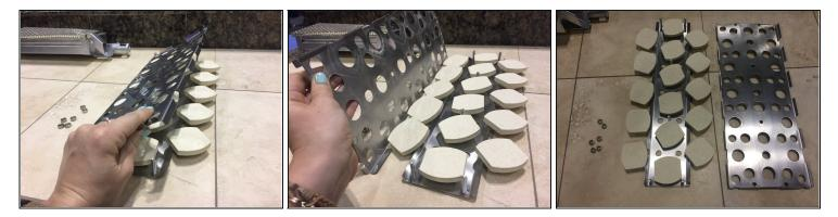
• Separate the front and back metal casings surrounding the briquettes.
