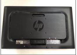
With the monitor laying flush against a table remove the 12mm 1cm head screws using a PH1 bit.
