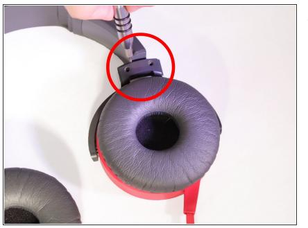
Now that the screws have been removed, pull away the plastic casing that covers the swivel piece (directly above the speaker).
