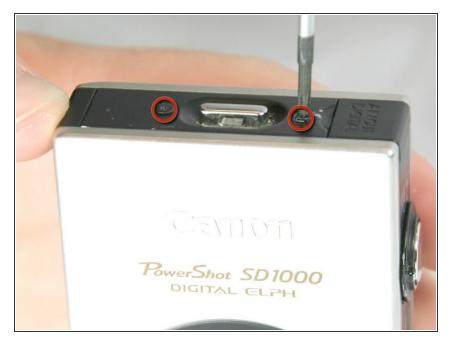
Remove the two 2.9 mm screws from the side panel farthest from the lens.
