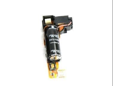
Pull the flash assembly forward out of the camera to remove it.
