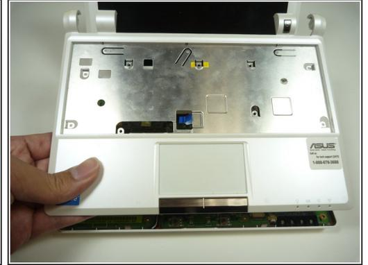
**⚠ Caution:** To clear the audio and microphone, lift the right half and move the cover to the left (as shown in the second picture) to prevent cover damage.
