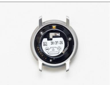
Pry the CR2025 lithium battery off and ponder the meaning of three hexadecimal numbers on the information sticker.
