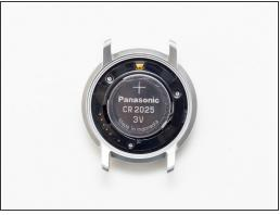
The case back can be opened by prying with the opening tool or a flat screwdriver. You will see the CR2025 lithium battery shining with all its glory.
