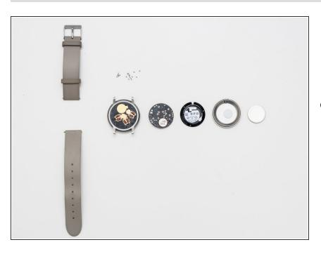
This Withings Activité Pop Smartwatch had water ingress and it failed due to corrosion. A common fault with this watch is loose inner screws, leading to poor PCB contact with motors. When you change battery make sure you apply silicone grease on the rubber gasket of the case back. The dial and hands are not accessible since the glass is pressed.
