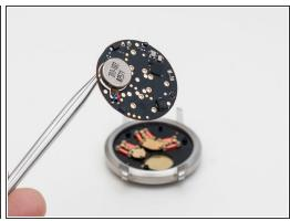
Using a thin flat blade screwdriver remove 12 (!) fine threaded screws to release the main PCB from the stepper motors of three dial hands.
