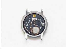
Using a thin flat blade screwdriver remove three self tapping screws holding the inner plastic cover.
