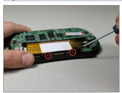
Unscrew the 2 Philips #00 screws on each side of the charging port.
