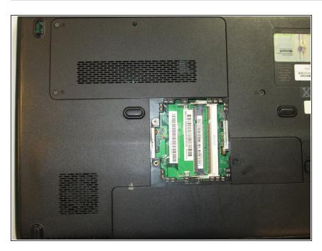
Remove each one of the rams so that the computer looks like this. You can do so be squeezing tabs on each side of the ram.
