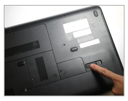
Push this slide over in order to remove the battery. This is safe when working with your computers memory.
