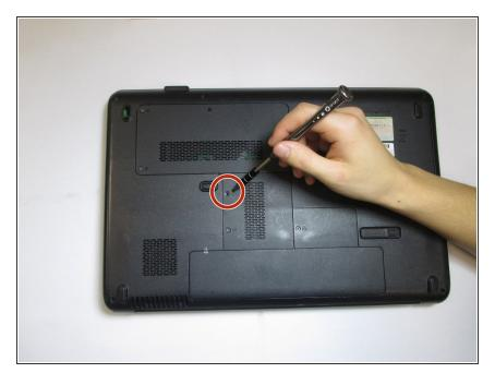
Lay the computer so that the backside is facing you and locate the screw in the picture.
