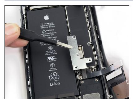
• Remove the lower connector bracket.
