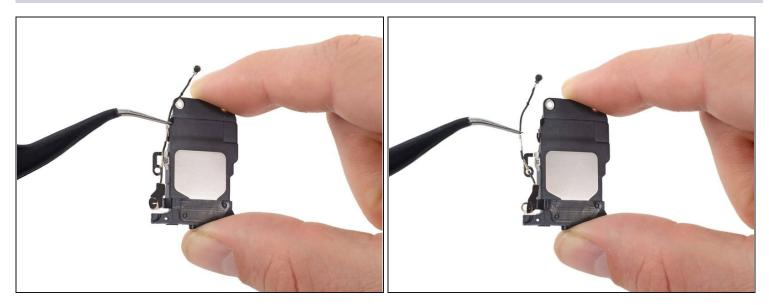
• Gently remove the antenna from the clip on the speaker.
