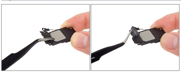
• Gently remove the tab by lifting up with tweezers and separate the tab from the speaker.
