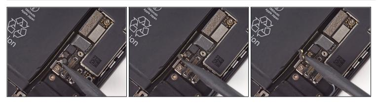
• Use the point of a spudger to lift the two antenna cable connectors up off of the sockets on the logic board.
