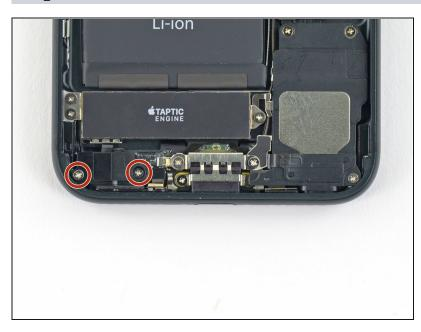
• Remove the two 1.9 mm Phillips screws securing the barometric vent to the rear case.
