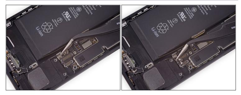
• Use tweezers to derout the antenna cables from their bracket on the logic board.
