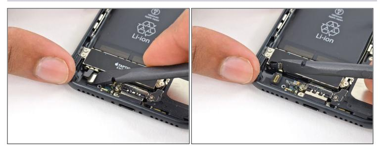
• Use the flat end of a spudger to disconnect the Taptic Engine connector from its socket on the logic board.
