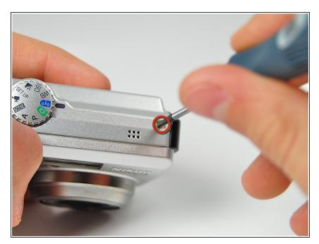
Remove the screw located near the speaker port using a Phillips 00 screwdriver.
