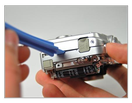
Using the plastic opening tool pry the back casing of the camera.
