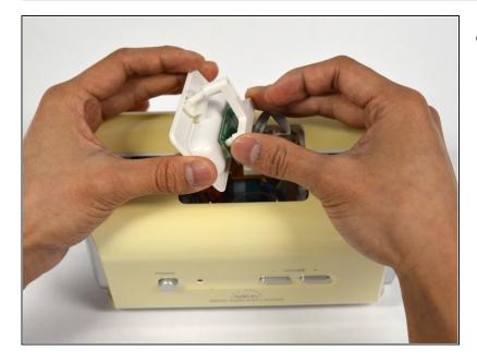
• Remove the T-shaped circuit board holder.
