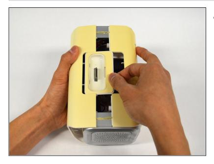
• Slide the dock connector out of the housing part.
