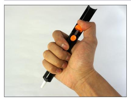
• Trigger the <u>desoldering pump</u> before heating the solder.
