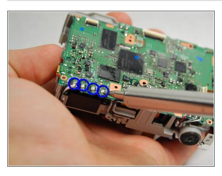
Carefully de-solder the four connections to the motherboard.
