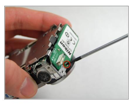
Remove the screw holding the Wifi Card to the camera body.
