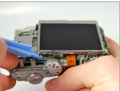
Use plastic opening tool to carefully pry the LCD Screen from the camera.
