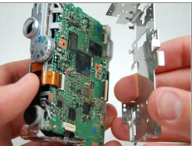
Carefully remove the back housing body from the camera.
