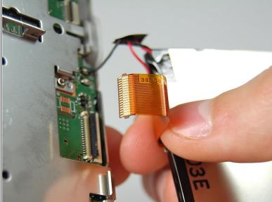
Gently pull the ribbon cable down to release the latch, then pull up to remove it from the motherboard.
