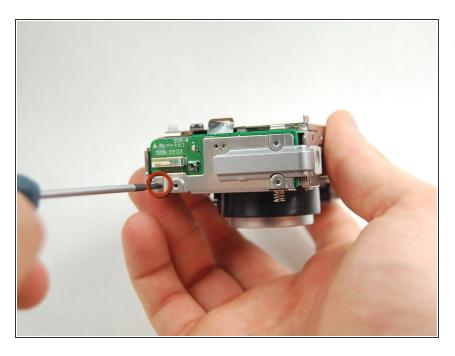
Remove the final screw connecting the Wifi card cover to the case.
