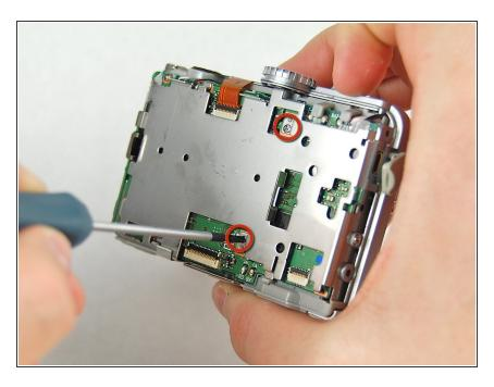
Continue by removing two screws from the back of the camera body.
