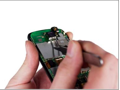
Using a pair of metal tweezers, simultaneously depress both tabs on one side of the camera enclosure and gently pull up until tabs come free. Repeat for the opposite side.
