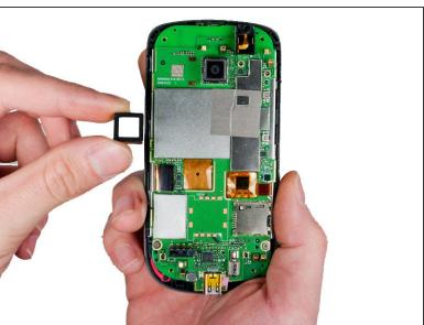
Pull the released camera enclosure away from the motherboard until it is completely free.
