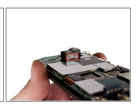
Locate the four metal tabs on the top and bottom of the camera holding the camera enclosure to the motherboard.
