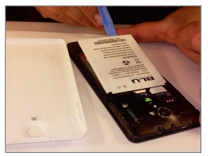
Remove the battery from the phone with the plastic opening tool, or your fingers.
