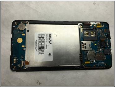
• Remove the bottom inner back plate.
