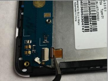
• Holding the cable with the removal tool, gently pull in the direction of the cable to remove the connector from its socket.
