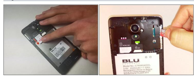
• Remove the microSD and SIM card. Gently tug on the microSD and SIM card to slide them out of their insert.
