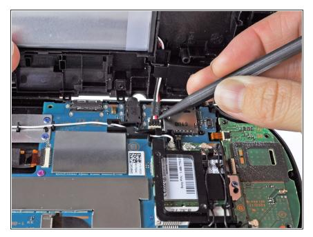
Free the battery cable by gently prying up on the connection with a spudger.
