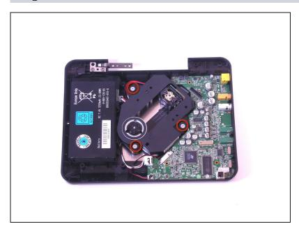
• Remove Philips screws with the #0 Philips Screwdriver.
