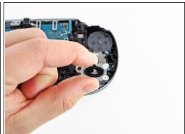
Using tweezers, peel up and remove the PS button.
