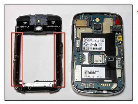
The two antennas are built into the rear case. Replace this piece to replace the antenna.
