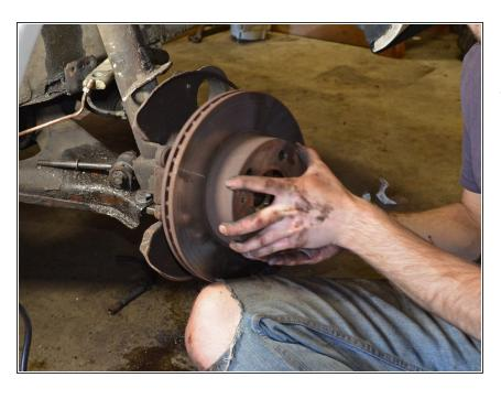
Pull the brake rotor straight off the wheel lugs to remove it.
