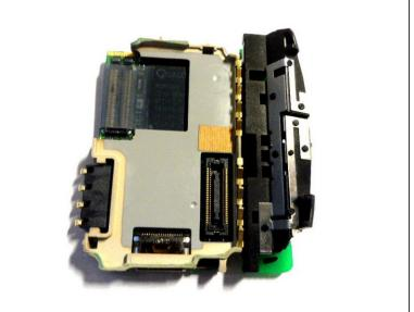
After the connection is removed, the motherboard is successfully removed.
