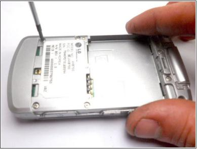
Remove the nine 4 mm screws from the back cover with a Phillips #0 screwdriver.
