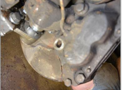
Use a 15 mm box end wrench to remove the two bolts on the back of the brake caliper.
