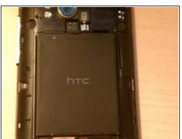
First pry the battery cover off of the back of the phone
