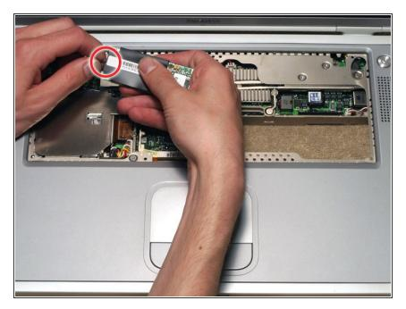
Disconnect the connector cable from the modem.
