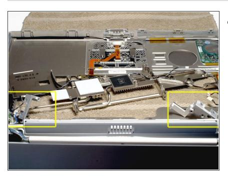
Lift up the metal brackets on either side of the upper case.
