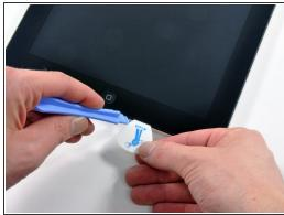
Some <u>heat</u>, <u>guitar picks</u>, and a plastic opening tool make <del>quick</del> arduous work of <del>removing</del> budging the front panel.
