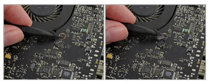
• Use a spudger to pry the fan connector straight up off the logic board.
