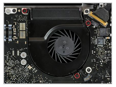
Remove three 3.5 mm Phillips screws securing the left fan to the upper case and logic board.
