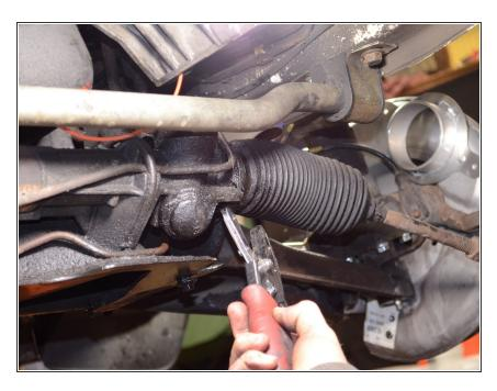
Use a pair of pliers to remove the zip tie or clamp securing the inner tie rod boot.
