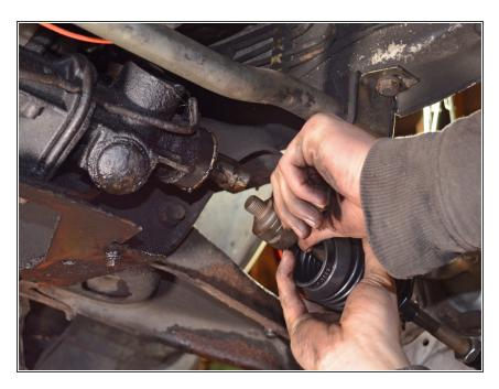
Install the inner tie rod end into the steering rack and tighten it with groove joint pliers.
