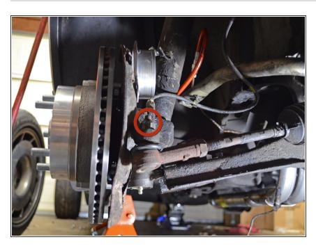
Use an impact wrench to remove the 19 mm tie rod end nut near the brake rotor.
