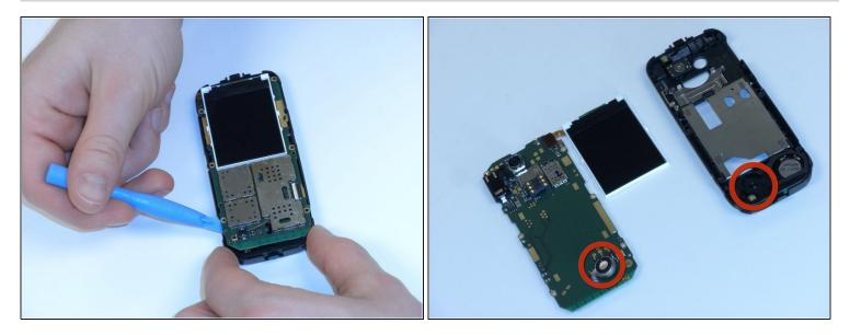
• Using the plastic opening tool, gently pry off the motherboard from the plastic shell. Place the metal display in a safe location for reassembly.
