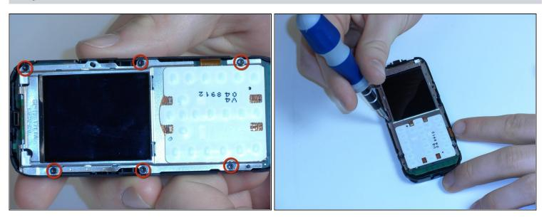
• Remove the six screws along the edges of the phone using a Torx 5 screwdriver.
