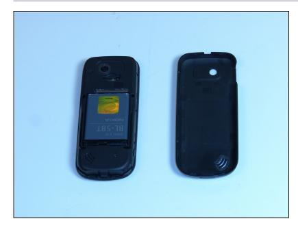
Remove the back cover to expose the battery. Put the plastic cover in a safe location for later.
