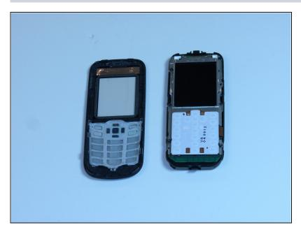
• Remove the faceplate with the number pad attached and put the faceplate to the side.
