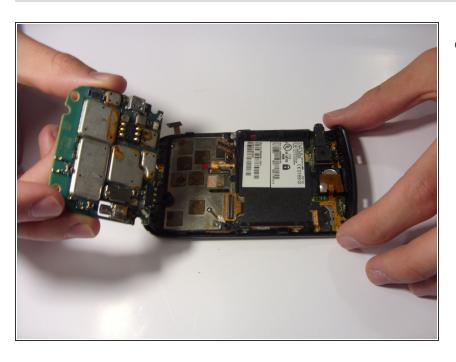
Remove the mother board by lifting the board upward.
