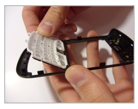
Lift the keypad out of the the front cover. To reassemble your device, follow these instructions in reverse order.
