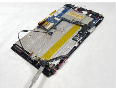
Carefully lift the I/O Board off the device.
