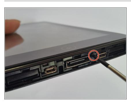
Remove the five 4 mm screws from the edges of the tablet with a Phillips #00 screwdriver.
