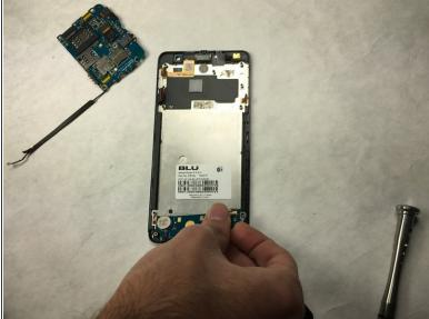
Peel off the bottom back with finger or supdger.
