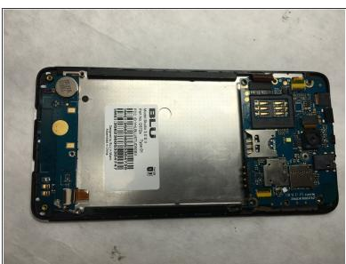
Remove the bottom inner back plate.
