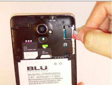
Remove the microSD and SIM card. Gently tug on the microSD and SIM card to slide them out of their insert.
