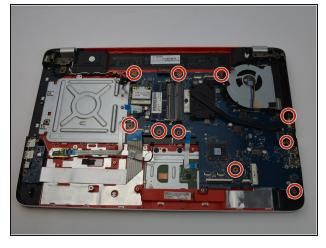
Remove the 7mm screws holding down the motherboard to the frame.
