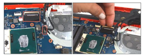
• Where the CPU fan was, lift the securing tabs on the cables and extract them from the motherboard.
