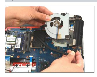
• Lift the fan out and then lift out the black grill covering the processor.
