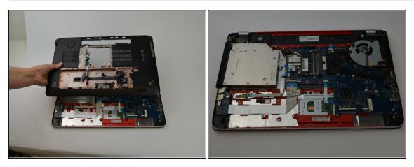
• Pull the under panel from the laptop by pulling at the edges once all screws are removed. Gently lift it off and place to the side.
