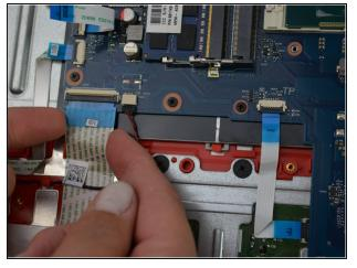
On the left side of the motherboard, remove the two cables by first lifting the black secure tabs and using the translucent tabs to pull them out.
