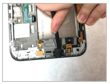
Using a nylon spudger, or any flat tool, gently pry and lift the small rubber covering to expose the auxiliary port.
