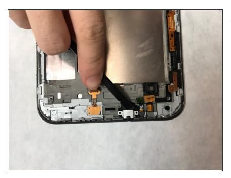
Using a nylon spudger, or any flat tool, gently pry and lift the small metal covering off of the auxiliary port.
