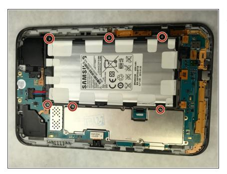
Using a Phillips head screwdriver, remove the 6 4mm screws holding holding the battery on the device.
