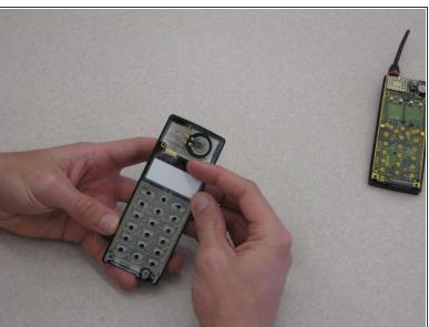
After removing the battery casing and taking apart the phone casing, the keypad is held in with a
