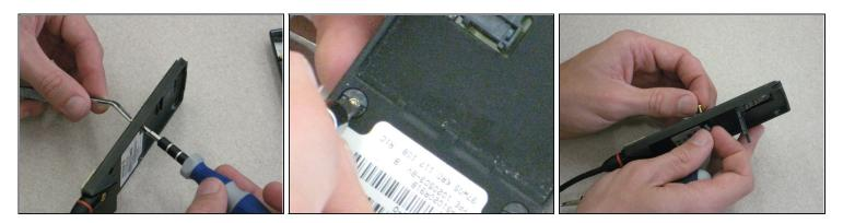
• Using the SP2.6 u-shaped screw driver in one hand, loosen and remove both center screws. Hold the back part of the screw with the metal <u>tweezers</u>.
