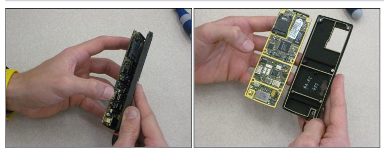
• With one hand on the circuit board and one hand on the phone casing, carefully pull apart the circuit board from the front panel casing.
