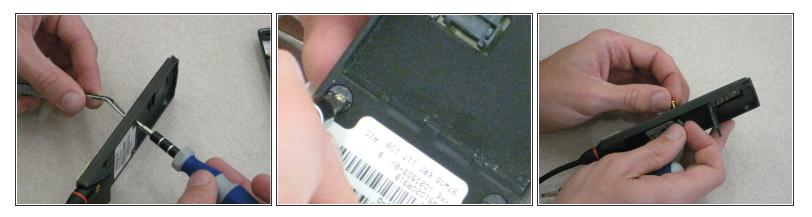
• Using the SP2.6 u-shaped screw driver in one hand, loosen and remove both center screws. Hold the back part of the screw with the metal tweezers.
