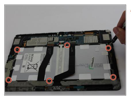
Remove the six 3mm screws around the battery with the <u>Phillips PH000</u> <u>screwdriver</u>.
