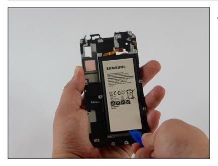
• Insert a plastic opening tool on the side of the frame and pull out the battery.
