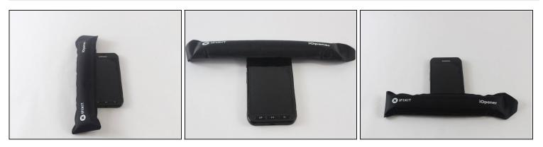
• Heat the front face (sides, top, bottom) of the phone with the iOpener, a hair dryer, or a heat gun for 60 seconds to loosen the adhesive around the edge of the glass.
