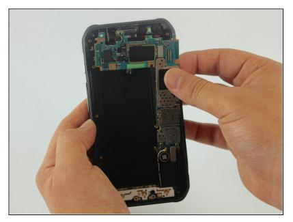
• Remove the motherboard from the rear case.
