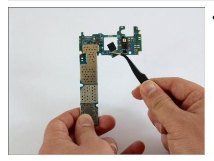
• Use the <u>tweezers</u> to remove the front camera from the motherboard.
