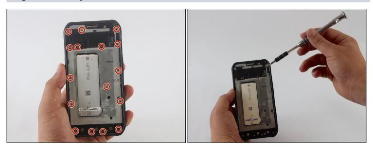
• Use the Phillips Head Screwdriver sized PH000 to remove the sixteen 4mm screws from the frame.
