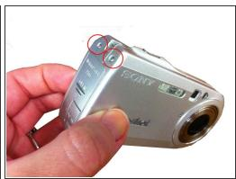
First locate the appropriate screws for detachment.
