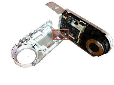
Carefully separate the front casing from the camera body.
