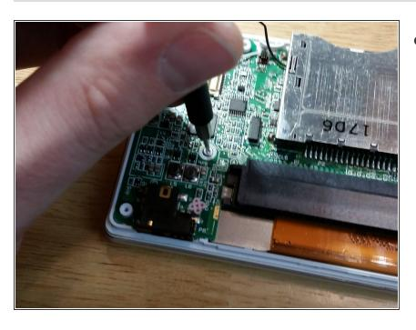
Remove the final screw holding down the motherboard.
