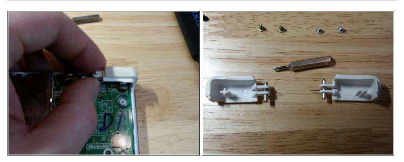
Carefully grasp and remove the shoulder buttons. Try to hold the spring assembly together so that you don't lose any pieces. The spring wire can puncture your skin so exercise caution. Wear safety glasses to avoid any rogue springs!
