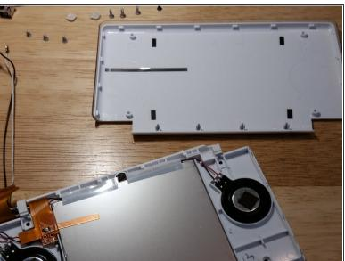
• With the plastic spudger, pry the top cover loose. Do not remove or otherwise mess with the rubber pieces on the side. You never need to touch those, and I've seen them unnecessarily damaged and missing countless times. As noted in the comments, the screen will slide down a millimeter or two, allowing the pieces to separate easily.
