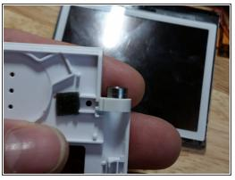
• If the flex cable is damaged, then you're out about \$8 as of this writing. Exercise extreme caution with this fragile piece, carefully rolling it into a tight cylinder. If the flex cable is damaged, there is no way to repair the LCD, and the entire module must be scrapped. Remove and set aside the metal piece.
