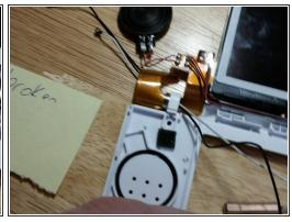
Noting the routing of the black and white wires for later reassembly, remove the microphone and Wi-Fi antenna, carefully pulling the wires through the center of the flex cable so as not to cause any damage.
