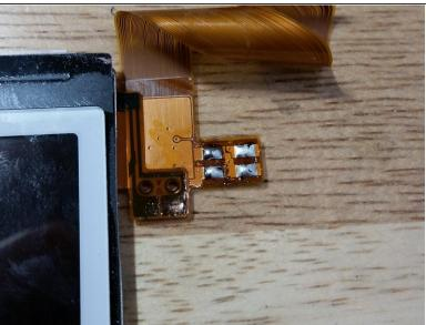
Clean up the contacts as you prefer. I use a tiny American-made solder wick and I've applied some fresh lead-based solder.
