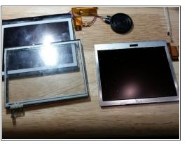
Slide the metal spudger under the black sticker and carefully work your way around the assembly, avoiding the flex cables. This step is easier than it looks, but only perform this step if the screen or the digitizer needs to be replaced. If both are functional, this step is unnecessary. Thoroughly clean both pieces with alcohol afterwards.
