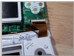
Flip the motherboard around as shown. Be gentle as the flex cable is fragile. Note the Chinese writing on the console made at the Nintendo factory.
