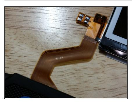
Inspect the flex cable for damage.
