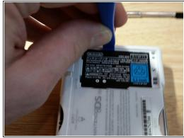
Unscrew the battery case with a PH000 bit. You will probably need to pry open the battery case as
