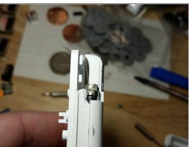
This is the chief design flaw of the Nintendo DS Lite. The latch assembly is much too fragile. Save the screws and the metal and plastic piece if you're replacing the shell.
