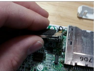
You must remove the Wi-Fi daughterboard at this stage or you risk damaging the digitizer. I learned this the hard way. You will need to pull hard on the daughterboard as the adhesive is very strong. You can try using heat or alcohol could to loosen the daughterboard, but that could risk damage to the components and I've never needed to do it.
