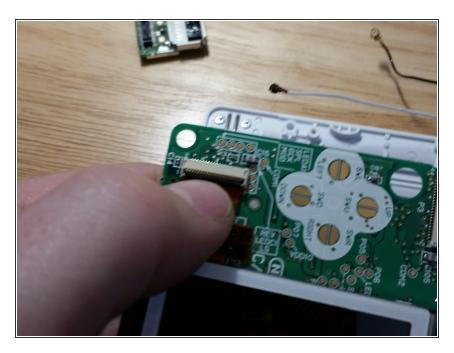
Remove the lower display flex connector. Pry the clip up with your fingernail, as you did with the upper display.
