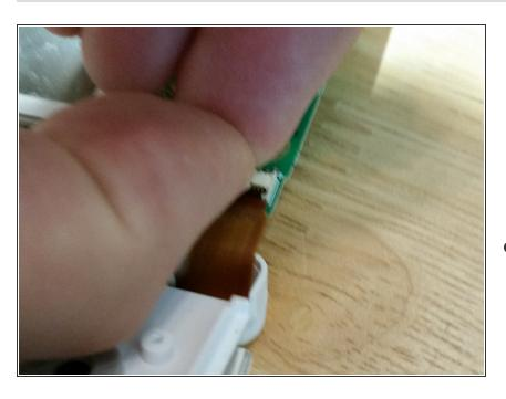
Remove the flex cable with your fingernail. Do not use a flathead bit, as it may damage the connector.
