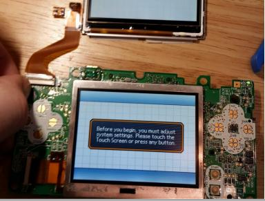
Optional: Test the disassembled unit. First, connect the Wi-Fi daughterboard. Connect the two screens, excluding the digitizer. While holding the battery in place, turn on the unit. Be cautious if you have removed any insulating material and there is new exposed metal. It is possible to blow a fuse or cause worse damage.
