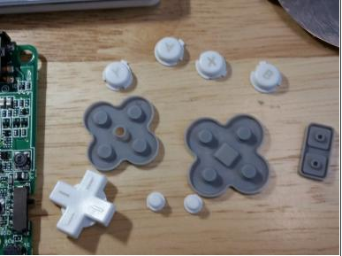
Remove the rubber and plastic button assemblies. This step is pretty easy, but don't lose any pieces. Every plastic and rubber piece can immediately go into hot, soapy water. Replace any rubber piece that is torn or excessively damaged.
