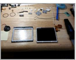
• The plastic cover is wedged underneath the back metal cover and is held on by a few different schemes, depending upon how old the DS Lite is. One method is two tabs on each side. Gently work the tabs loose without removing the back metal cover. This step is unnecessary unless you're changing the color of the shell.
