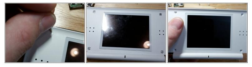
• With the smallest flathead bit you can find, work the bit under the sticker to avoid damaging the unit as much as possible. Slightly marring the ABS plastic is nearly impossible. I've had luck more recently using a plastic razor blade.
