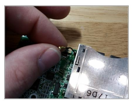
Remove this black wire. You will have to wiggle it out. One of the stupidest design decisions on the DS Lite besides the latch problem, the black wire is even harder to put back in. Do not attempt to mess with the DS cartridge port in any way. With persistence, the black wire will come out and it will go back in when the time comes.
