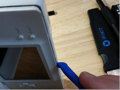
• I see a lot of damage caused by carelessly removing the bottom cover, so take your time and carefully move the plastic spudger around the perimeter. If the bottom cover seems glued on, remove the cover with the unit closed. This may help prevent scratching the digitizer.
