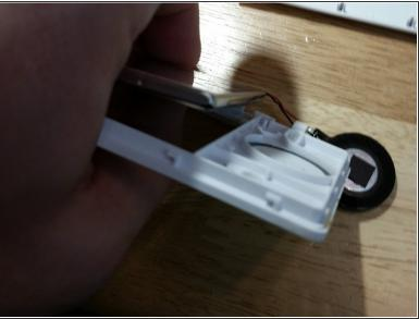
Begin pressing on the top screen as show here and work your way around. Be fairly gentle but note that the actual LCD is protected by a plastic shield in front and a metal shield in back.
