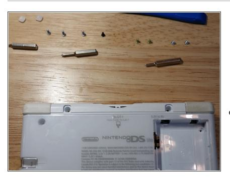
Now remove the two gold colored screws under the rubber feet and the two silver colored screws in the battery compartment with the PH000 bit. Then remove the three silver
