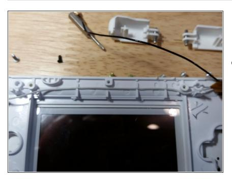
The most common reason why DS Lites don't go together properly is that this white wire is not routed properly. When reassembling, follow this routing scheme and the finished product will feel like it is fresh off the factory floor.
