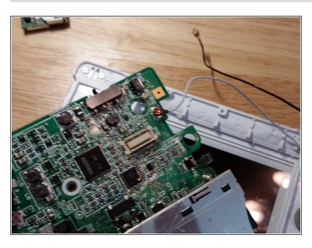
• Make note of how the white wire is routed. You will need to replicate this routing for the reassembly. Now remove the white wire. Make sure that the digitizer flex cable was detached earlier. If not, go back and perform this step.
