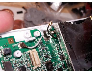
Gently lift the digitizer flex connector from this side with a small flathead bit. Take your time and be gentle as this connector is easily broken. Replacing the digitizer is an extremely common repair for this console so I highly recommend learning how to do this.
