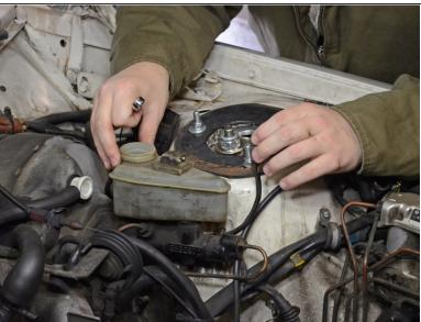
If your brake fluid reservoir has a fluid level sensor, disconnect it by pressing down on the plastic tab and pulling the connector straight out of its socket.
