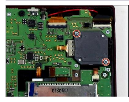
• Using a JIS #000 screwdriver, remove the two 8 mm screws securing the circle pad.
