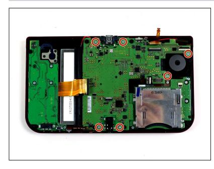
• Using a JIS #000 screwdriver, remove six 4mm screws along the edges of the motherboard.
