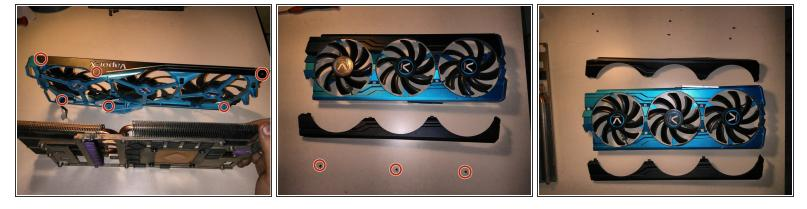
Remove 3 screws per side (6 screws in total) to release the 2 metal plates
