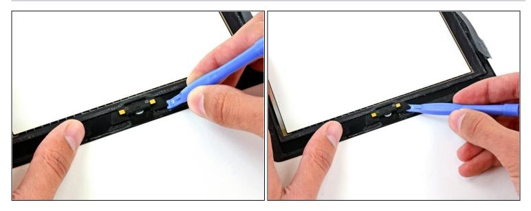
• Wedge the plastic opening tool under the right side of the home button assembly and pry upwards, releasing the adhesive on that side.
