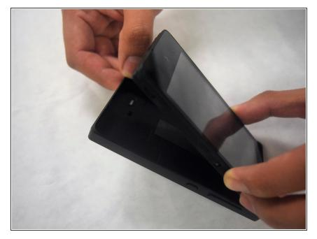
Remove the back cover of the device by applying light pressure toward the outer rim and display.
